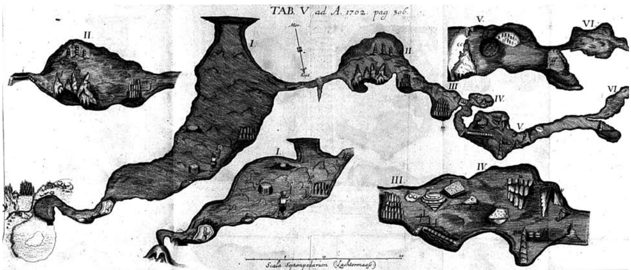
Figure 4. This map of the Baumann's Cave was published as a copper etching by V. D. HARD in the "Acta eruditorum", 1702. The map is oriented to the south and has already a north arrow and a scale (in Harzer Lachter; 1 HL = ca. 2 m). There is a plan view and four longitudinal sections of certain parts of the cave. The letters refer to the individual flowstone formations shown to the visitor (For details see KEMPE et al. , 2004. (Original: collection Kempe).
