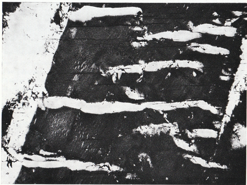
Fig. 1. Microphotograph of specimen S 478 (cf. Fig. 3), Eganville, Ontario. Section parallel to (010); crossed nicols; 48\times . Plate albite is visible parallel to the cleavage traces of (001). Vein albite (thick) and film albite (thin) are also visible nearly vertical, and parallel to the c -axis direction. The albite appears white.
